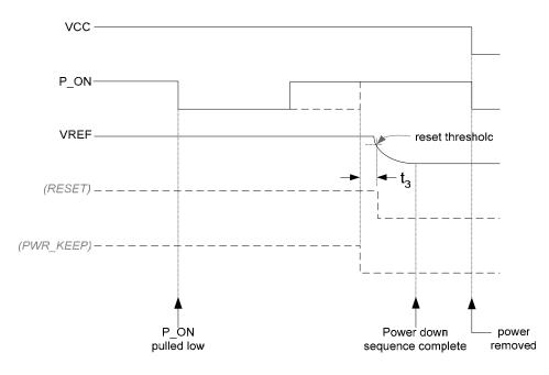
Figure 5.8–3 Power Down timing
